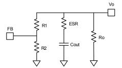
Figure 8—Simplified Circuit in skip Mode
