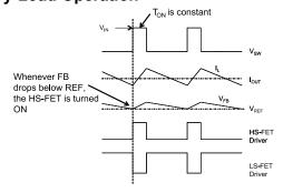
Figure 2—Heavy Load Operation
