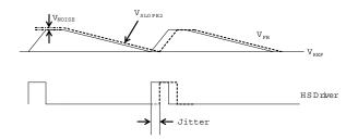
Figure 5—Jitter in Skip Mode
