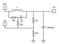
Figure11—Simplified Circuit of Ceramic Capacitor
