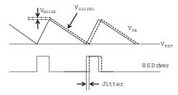
Figure 4—Jitter in PWM Mode
