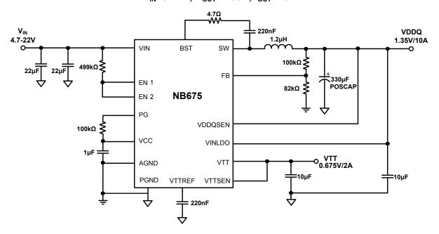
Figure 15 — Typical Application Circuit with Large ESR POSCAP Output Capacitor  $V_{\text{IN}}$ =5-22V,  $V_{\text{OUT}}$ =1.35V,  $I_{\text{OUT}}$ =10A
